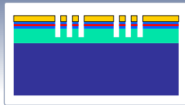
PhC etching (ICP \text{Cl}_2/\text{N}_2 )
