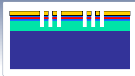
PhC etching (ICP \text{Cl}_2/\text{N}_2 )
