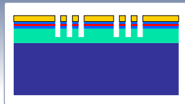
PhC etching (ICP \text{Cl}_2/\text{N}_2 )
